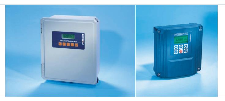
Up to four cooling circuits or boilers can be controlled simultaneously by the AQUATRAC<sup>®</sup> cooling tower control. It can perform all the requisite functions, including bleed control, metering of two biocides and inhibitors, as well as monitoring of the entire process. Cooling tower control can be performed in conductive or volumetric mode.
